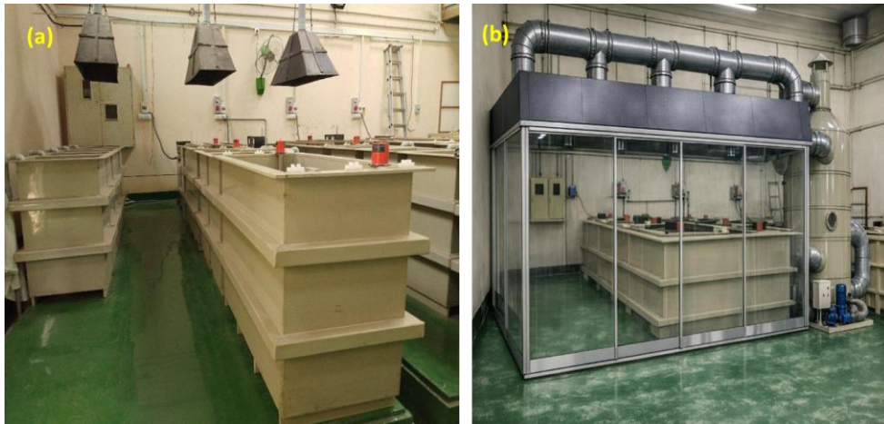
Figure 1. (a) Typical electroplating process tanks, without extended fume hood design (b) Modified design for the Fume hood.
